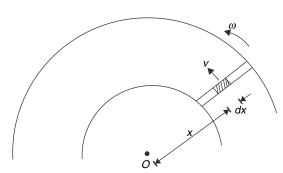
Consider an element of length dx on the blade. Speed of this element is  $v = \omega x$  Viscous force on this element is
