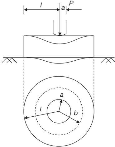
$a$  = Radius of contact between road and tyre
