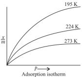
These curves indicate that on increasing temperature, physical adsorption decreases at a fixed pressure.
