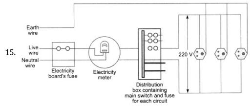
A fuse in a circuit prevents damage to the appliances and the circuit due to overloading. Otherwise, the appliances or the circuit may be damaged.
