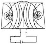
Here the current is passing clockwise when looked from front side. At the points where the conductor passes through horizontal plane, the lines of force are almost circular, their direction being given by right-hand grip rule. Near the central region, the lines are quite straight and at right angles to the plane of the coil.
