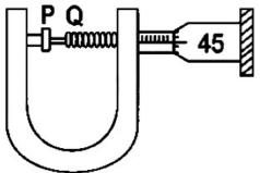
(A) Screw moves 0.5 mm on main scale in one complete rotation
