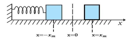
Consider a spring oscillating between  $-x_m$  and  $x_m$  . At any point x between  $-x_m$  and  $x_m$  , the total mechanical energy of the spring
