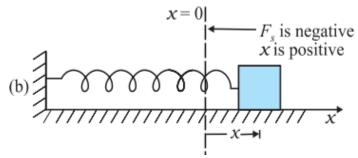
Consider a block of mass m attached to a spring and resting on a smooth horizontal surface. The other end of the spring is attached to a rigid wall. Let the spring be pulled through a distance x.
