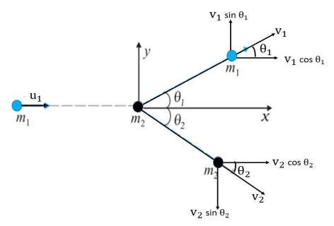
Consider the elastic collision of a moving mass  $m_1$  with the stationary mass  $m_2$ .
