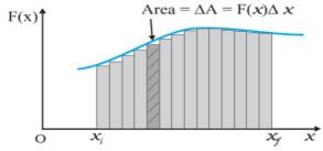
If the displacement  $\Delta x$  is small, we can take the force F (x) as approximately constant and the work done is then
