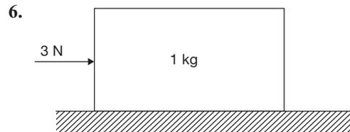
A body of mass 1 kg is resting on a plane surface as shown in the figure. A force of 3 N is gradually applied on one side as shown. Coefficient of static friction is 0.35 and coefficient of kinetic friction is 0.3. The friction force acting is
