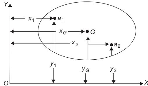
The above figure shows an irregular lamina of total area 'A' whose centre of gravity is to be determined. Let the lamina be composed of small areas  $a_1, a_2, \dots$ , etc., such that:
