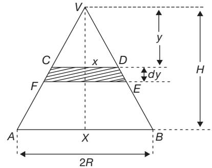
Consider one such disc of radius  $x$ , thickness  $dy$  and at a depth  $y$  from the vertex of the cone, i.e., from  $V$ .
