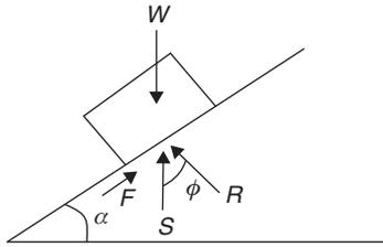
The above figure shows a block of weight  $W$  on a rough inclined plane which is inclined at an angle  $\alpha$  with the horizontal. Let  $R$  be the normal reaction and  $F$  be the force of friction. From applying the condition of equilibrium, algebraic sum of the forces resolved along the plane:
