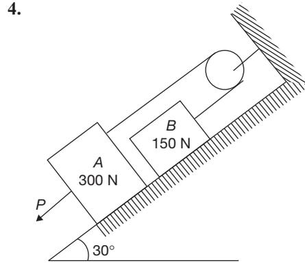
Two blocks  $A$  and  $B$  weighing 300 N and 150 N respectively are placed on a rough inclined plane of angle  $30^\circ$  and connected through a string over a pulley as shown in the figure. Coefficient of friction of the contact surfaces are 0.25. Force  $P$  required on block  $A$  for impending motion of the blocks is
