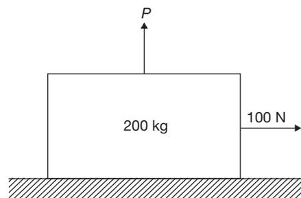
A body of mass 200 kg rests on a horizontal surface as shown in the figure. Coefficient of friction between the body and surface is 0.2. If a horizontal pull of 100 N can be exerted on the body, the vertical force  $P$  required to move the body is
