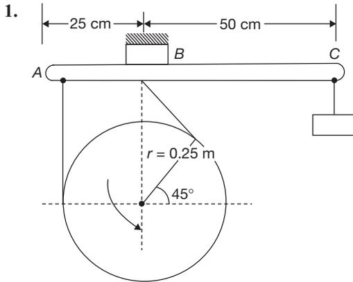
A rotating wheel is braked by a belt  $AB$  attached to the lever  $ABC$  hinged at  $B$ . The coefficient of friction between the belt and the wheel is 0.5. The braking moment exerted by the vertical weight  $W = 200$  N is
