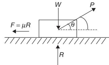
Force ' $P$ ' is applied, at an angle  $\theta$  to the horizontal, on a block of weight  $W$ , such that the motion impends or the block tends to move.
