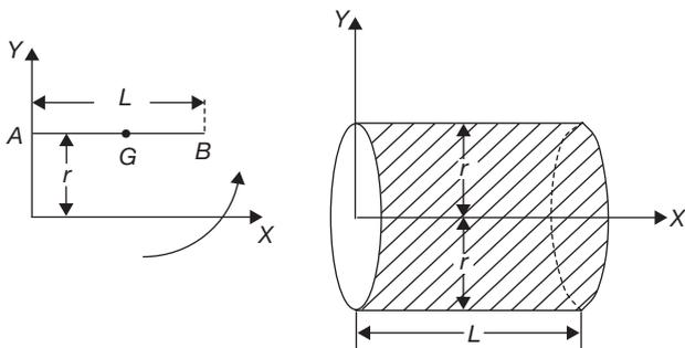
For example, in the above figure, the curved surface of a cylinder is obtained by rotating the line  $AB$  about the  $X$ -axis.
