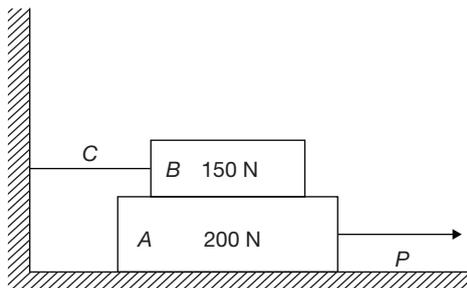
Block A weighing 200 N is placed on plane floor and block B weighing 150 N is placed over block A. Block B is constrained by a string  $C$  and a force  $P$  is applied on block A as shown in figure. For the contact surfaces, coefficient of static friction is 0.3 and coefficient of kinetic friction is 0.25.
