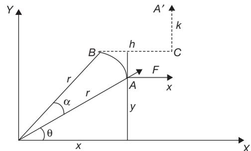
To illustrate the principle of work, let us consider a body at equilibrium at a point  $A$ . A force ' $F$ ' acts on the body and displaces it to the point  $A'$ , where the displacement consisting:
