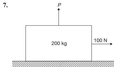
A body of mass 200 kg rests on a horizontal surface as shown in the figure. Coefficient of friction between the body and surface is 0.2. If a horizontal pull of 100 N can be exerted on the body, the vertical force  $P$  required to move the body is
