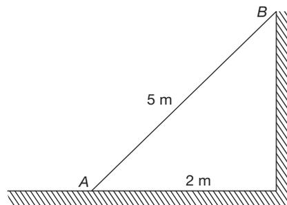
A uniform ladder of length 5 m and weight 250 N is placed against a smooth vertical wall with its lower end 2 m from the wall. Coefficient of friction between floor and ladder is 0.25. Friction at the wall may be neglected. Frictional force at A, the bottom of ladder is
