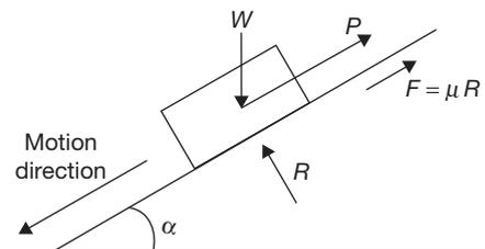
$$\boxed{\text{For motion down the plane, } P = \frac{W \sin(\alpha - \phi)}{\cos \phi}}$$
