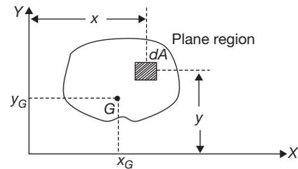
Let  $dA$  be a differential (i.e., infinitesimal) area located at the point  $(x, y)$  in the plane region area  $A$ .
