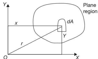
The moment of inertia of the area about the  $X$ -axis and  $Y$ -axis are
