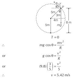
**Example 10.** A stone of mass 1 kg tied to a light in extensible string of length  $L = \frac{10}{3}$  m is whirling in a circular
