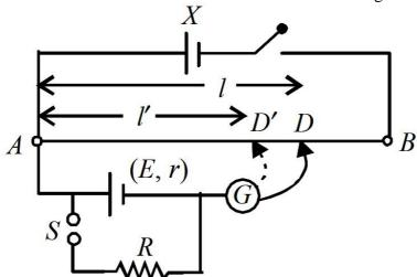
The terminal voltage V is now balanced against a smaller length AD' = l'.
