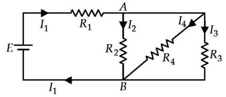
**Ans.** From figure,  $R_2$ ,  $R_3$  and  $R_4$  are connected in parallel.
