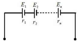
If n cells having emfs  $E_1$ ,  $E_2$ , ...,  $E_n$  and internal resistances  $r_1$ ,  $r_2$ , ...,  $r_n$  are connected in series as shown, then
