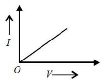
The **resistance** of a conductor is a measure of the opposition offered by the conductor to the flow of current. This opposition is due to frequent collision of the electrons with the atoms of the conductor.
