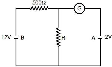
**Ans.** If galvanometer G gives zero deflection, than current of source of 12V flows through R, and voltage across R becomes 2V.
