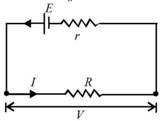
The resistance offered by the electrolyte to the flow of current through the cell is called the *internal resistance* of the cell.
