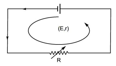
Suppose a current I flows through the circuit and using loop rule
