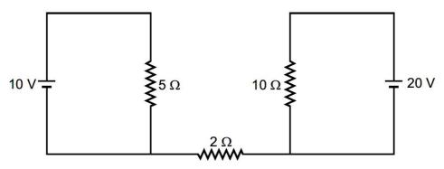
Ans. No current will flow through  $2\Omega$  resistor, because in a closed loop, total p.d. must be zero. So
