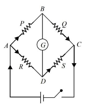
The measurement of resistance by Wheatstone's bridge is not affected by the internal resistance of the cell.
