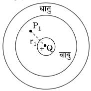
A small metal sphere carrying charge +Q is located at the centre of a spherical cavity in a large uncharged metallic spherical shell. Write the charges on the inner and outer surfaces of the shell. Write the expression for the electric field at the point  $P_1$ .
