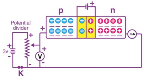
p-n Junction diode in forward biased
