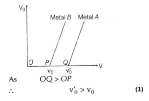
So, the threshold frequency of metal A is greater than metal B.
