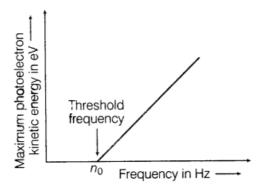
(i) Planck constant is given by slope of the curve, i.e. as
