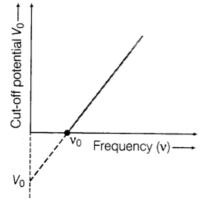
From this graph, we can calculate the value of threshold frequency (point of intersection of frequency axis) and stopping potential (point of intersection on potential axis).
