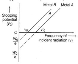
**Ans.** Metal A has higher value of work-function because and the intercept of the line of the given graph depends on work-function.
