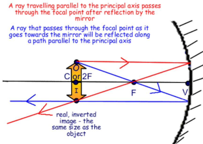
When the object is placed on the center of curvature in front of the concave mirror, the rays parallel to the principal axis pass through the focus. Another incident ray which passes through the focus after reflection will be parallel to the principal axis. The two reflecting rays meet at the center of curvature, thus an image is formed there.
