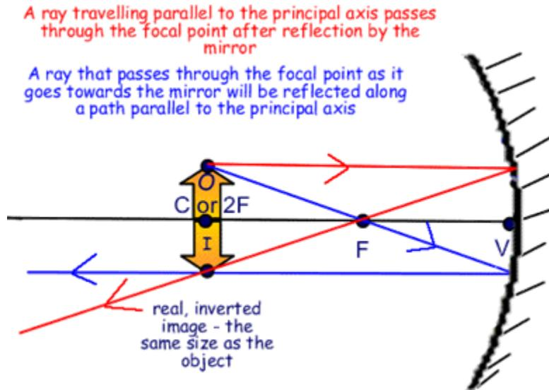
**Q. 22. Show the formation image with a ray diagram when an object is placed on the principal axis of a concave mirror away from the center of curvature. (AS5)**
