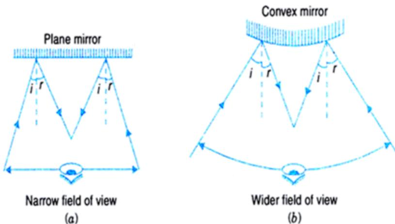
**Q. 30. A convex mirror with a radius of curvature of 3m is tried as rear view in an automobile. If a bus is located at 5m from this mirror, find the position, nature and size of the image. (AS7)**
