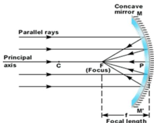
Focus is the point where the incident parallel rays converge, after reflection from the mirror, at a distance of  $R/2$  from the mirror where  $R =$  radius of curvature. Focal length is defined as the image distance when the object is at infinity.
