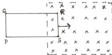
Mark the direction of induced current in the coil PQRS. State the rule used to find the direction of induced current. What would be the direction of induced current if the direction of magnetic field is reversed?
