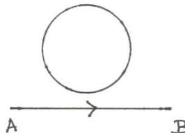
The figure shows a circular coil and a conductor  $AB$  carrying current from  $A$  to  $B$ . If the current is i) decreasing ii) increasing find the direction of induced current in the circular coil.
