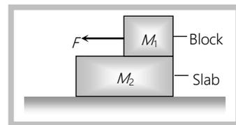
29. In the above problem if  $F = 100 \text{ N}$ , what will be the acceleration with which the slab will move
