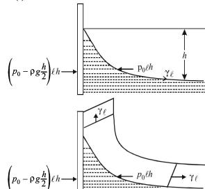
Balancing forces in horizontal direction
