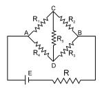
When current through the galvanometer is zero (null point or balance
