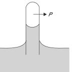
Force due to air pressure inside the tube  $\pi r^2 P(\uparrow)$ Force due to atmospheric pressure =  $\pi R^2 P_o(\downarrow)$
