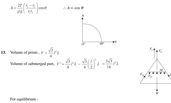
Spring force  $(F_S)$  + Buoyancy  $(F_B)$  = weight (W) + surface tension force  $(F_{ST})$
