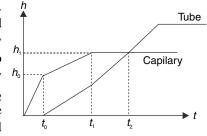
tube, the meniscus gets convex. After time  $t_2$  water begins to flow out of the capillary and water level in both tubes becomes constant.
