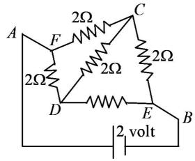
Now it is a balanced wheatstone bridge. The potential at point C and D is the same. No current flows between C and D.
