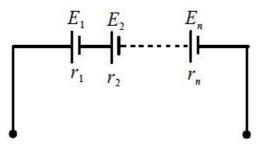
If *n* cells having emfs  $E_1$ ,  $E_2$ , ...,  $E_n$  and internal resistances  $r_1$ ,  $r_2$ , ...,  $r_n$  are connected in series as shown, then
