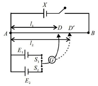
First the key  $S_1$  is pressed which brings  $E_1$  in the circuit. The sliding contact D is moved till the galvanometer shows no deflection. Let the length  $AD = l_1$ . Next  $S_1$  is opened and  $S_2$  is closed. This brings  $E_2$  in the circuit. Let D' be the new null point and let  $AD' = l_2$ . Then, clearly,
