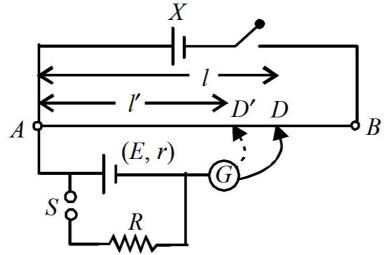
The terminal voltage V is now balanced against a smaller length AD' = l'. Then,  $\frac{E}{V} = \frac{l}{l'}$ But we know that  $\frac{E}{V} = \frac{R+r}{R}$
