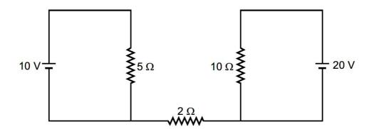
Ans. No current will flow through  $2\Omega$  resistor, because in a closed loop, total p.d. must be zero. So
