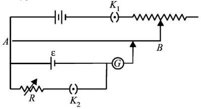
Initially key  $K_2$  is off Then at balancing length  $l_1$  $e = Kl_1$  ------ (i)
