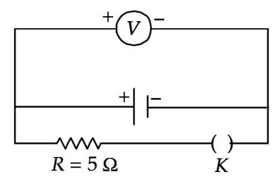
Later when *K* is closed, voltmeter reads 1.8 V which is actually the terminal potential difference, *V*. *i.e.* if *I* is the current flowing, then  $\varepsilon = I(R + r)$
