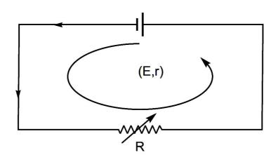
Suppose a current I flows through the circuit and using loop rule E - IR - Ir = 0
