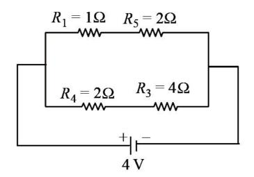
As  $R_1$  and  $R_5$  are in series, so their equivalent resistance is  $R' = R_1 + R_5 = 1 + 2 = 3 \Omega$ As  $R_4$  and  $R_3$  are in series, so their equivalent resistance is  $R'' = R 4 + R 3 = 2 + 4 = 6 \Omega$ So, net resistance of the network is
