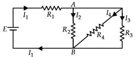
**Ans.** From figure,  $R_2$ ,  $R_3$  and  $R_4$  are connected in parallel.  $\therefore$  Effective resistance  $R_p$
