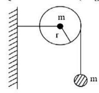
As shown in the figure, a bob of mass m is tied to a massless string whose other end portion is wound on a fly wheel (disc) of radius r and mass m. When released from rest the bob starts falling vertically. When it has covered a distance of h, the angular speed of the wheel will be:
