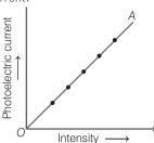
Using the incident radiations of a fixed frequency, it is found that the photoelectric current increases linearly with the intensity of incident light as shown in figure. Hence, a photocell employs photoelectric effect to convert change in the intensity of illumination into a change in photoelectric current.
