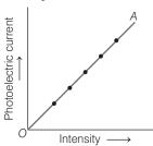
It means number of photoelectrons emitted per second from photosensitive plate is directly proportional to the intensity of the incident radiation.
