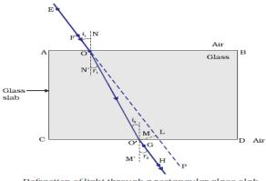
Refraction of light through a rectangular glass slab
