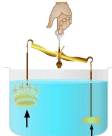
In water apparent weight of the crown is less than the apparent weight of pure gold.
