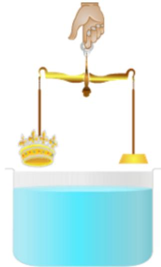
In air weight of the crown is equal to the weight of the piece of pure gold.
