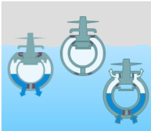
To raise the submarine, water is released from the tanks and compressed air (kept onboard in flasks) is let into them. The greater the amount of compressed air in the tanks, the higher does the submarine rise.
