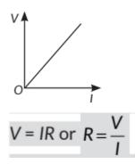
So, the slope of V-I graph at any point represents the resistance of the given conductor. As graph is a straight line, so it is clear from the graph that  $V \propto I$ .
