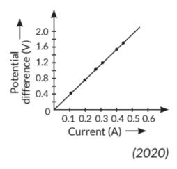
9. Study the V-I graph for a resistor as shown in the figure and prepare a table showing the values of (in amperes) corresponding to four different values V (in volts). Find the value of current for V=10 volts. How can we determine the resistance of the resistor from this graph? (Board Term I, 2016)
