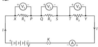
Given figure shows the series combination of three resistors  $R_1$ ,  $R_2$  and  $R_3$  connected across a voltage source of potential difference V. Let current I is flowing through the circuit.  $V_1$ ,  $V_2$  and  $V_3$  are the potential differences across resistors  $R_1$ ,  $R_2$  and  $R_3$  respectively. Since, the total potential difference across a combination of resistors in series is equal to the sum of potential difference across the individual resistors.
