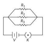
$$\frac{1}{R_{eq}} = \frac{1}{R_1} + \frac{1}{R_2} + \frac{1}{R_3}$$
