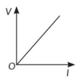
So, the slope of V-I graph at any point represents the resistance of the given conductor. As graph is a straight line, so it is clear from the graph that V I.
