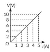
Hence, the value of current for V=10 volts is 5 amperes (or 5 A). From Ohm's law, V=IR,
