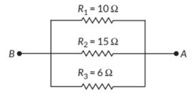
We know that 6  $\Omega$  and 4  $\Omega$  are in series, then  $R_1=6~\Omega+4~\Omega=10~\text{and}~3\Omega~\text{and}~3\Omega~\text{are in series,}~R_3=3\Omega+3\Omega=6Q~\text{Now}$  equivalent resistance between A and B,
