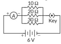
(a) Given, voltage of the battery = 2V + 2V + 2V = 6 V Current through 10  $\Omega$  resistance,
