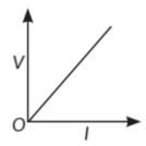
V-I graph for an ohmic conductor can be drawn as given in figure. Important feature of V-I graph are:
