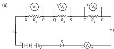
Given figure shows, the series combination of three resistors R<sub>1</sub>, R<sub>2</sub> and R<sub>3</sub> connected across a voltage source of potential difference V.
