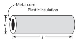
Plastic insulation surrounds a wire having diameter d and length I as shown above. A decrease in the resistance of the wire would be produced by an increase in the
