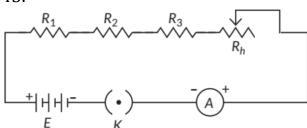
Change the positions of ammeter and note the reading of ammeter each time. You will find that all the reading obtained are same. So, the value of the current in the ammeter is the same, independent of its position in the electric circuit. It means that in this circuit (series combination) the current is the same in every part of the circuit. Precautions:
