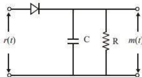
$r(t)$  is received signal and  $m(t)$  is message signal and for better reception RC must be selected such as
