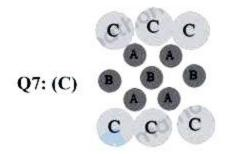
From figure, it is clear that 4 corners and 2 face centers lie on the shaded plane. Therefore, there will be six C atoms, and atoms (marked A) in TVs do not touch other.
