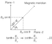
Let, plane 1 and 2 are mutually perpendicular planes making angle  $\theta$  and  $(90^{\circ} - \theta)$  with magnetic meridian. The vertical component of earth of earth's magnetic field remain same in two plane but effective horizontal components in the two planes is given by
