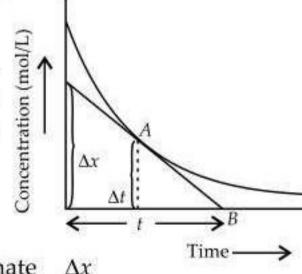
$$r_{\text{inst.}} = \lim_{\Delta t \to 0} -\frac{\Delta[A]}{\Delta t} = -\frac{d[A]}{dt}$$
