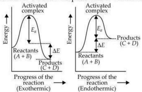
◆ Activation energy (E<sub>a</sub>) = E<sub>(activated complex)</sub> - E<sub>(ground state)</sub>  $\Delta H$  = activation energy of forward reaction - activation energy of backward reaction
