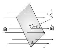
$\overrightarrow{B}$  at an angle  $\phi$  with the perpendicular to A: magnetic flux  $\varphi_{_{R}}=BAcos\theta$
