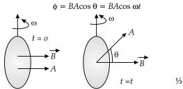
As the coil rotates, the magnetic flux linked with it changes. An induced emf is set up in the coil which is given by,
