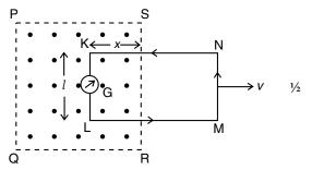
To calculate the emf induced, suppose in a small time  $\Delta t$ , the loop is moved out of magnetic field through a small distance  $\Delta x$ .
