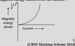
Q. 11. Derive the expression for the magnetic energy stored in a solenoid in terms of magnetic field B, area A and length l of the solenoid carrying a steady current I. How does this magnetic energy per unit volume compare with the electrostatic energy density stored in a parallel plate capacitor?
