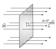
$\vec{B}$  parallel to A ( $\phi = 0^{\circ}$ ) magnetic flux  $\phi_B = BA$ .
