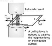
> Eddy currents flowing in a material will generate their own secondary magnetic field that opposes the coil's primary magnetic field.
