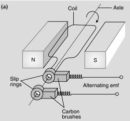
The AC Generator works on the principle of electromagnetic induction.
