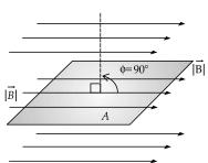
$\vec{B}$  perpendicular to A ( $\phi$ =90°): magnetic flux  $\phi_B$  = 0.
