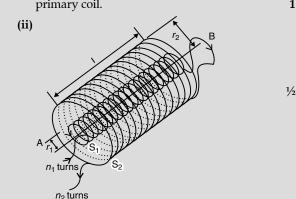
$\therefore B_2 = \frac{\mu_0 N_2 i_2}{l}$   $\therefore \text{ Flux linked with the primary coil}$   $= \frac{\mu_0 N_2 N_1 A_1 i_2}{l}$
