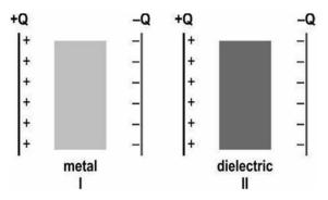
(a) Sketch the electric field lines between the plates in I and II.
