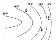
Using the relation between potential difference and electric field intensity, find which of the three points, A, B or C will have the greatest electric field intensity.
