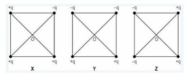
(a) Draw relevant vector diagrams to represent the resultant electric field ER at the center of the square in each case.
