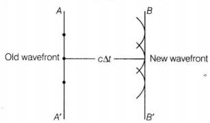
With these sources for the wavelets, we draw circular arcs, each of radius  $c \Delta t$ , where c is the speed of light in vacuum and  $\Delta t$  is some time interval during which
