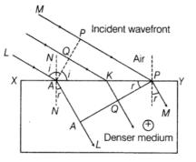
Suppose when disturbance from point P on incident wavefront reaches point P' on the refracted wavefront, the disturbance from point Q reaches the point Q' on the refracting surface XY. Since, A'Q'P' represents the refracted wavefront, the time taken by light to travel from a point on incident wavefront to the corresponding point on refracted wavefront should always be the same. Now, time taken by light to go from Q to Q' will be
