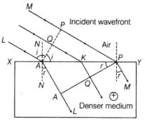
Suppose when disturbance from point P on incident wavefront reaches point P' on the refracted wavefront, the disturbance from point Q reaches the point Q' on the refracting surface XY. Since, A'Q'P' represents the refracted wavefront, the time taken by light to travel from a point on incident wavefront to the corresponding point on refracted wavefront should always be the same. Now, time taken by light to go from Q to Q' will be
