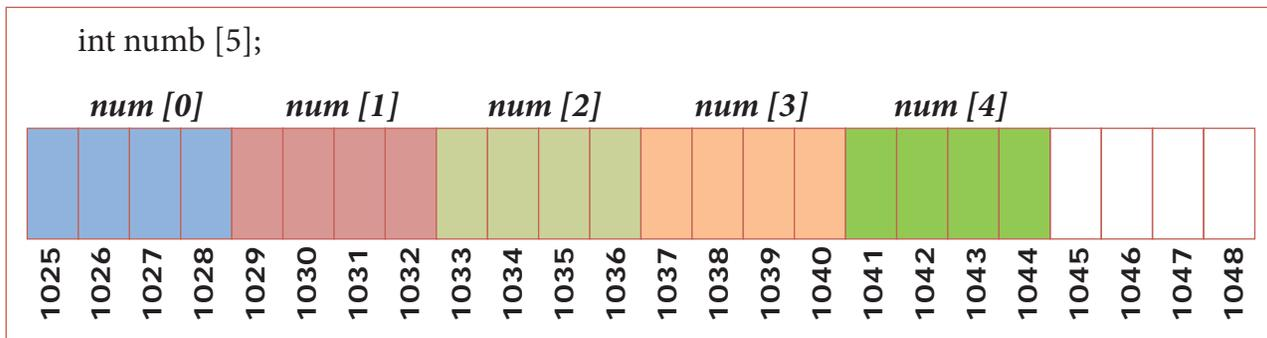
The above figure clearly shows that, the array num is an integer array with 5 elements. As per the Dev-C++ compiler, 4 bytes are allocated for every int type variable. Here, there are totally 5 elements in the array, where for each element, 4 bytes will be allocated. Totally, 20 bytes will be allocated for this array.
