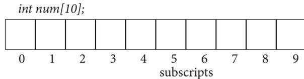
Each element (Memory box) has a unique index number starting from 0 which is known as “subscript”. The subscript always starts with 0 and it should be an unsigned integer value. Each element of an array is referred by its name with subscript index within the square bracket. For example, num[3] refers to the 4th element in the array.
