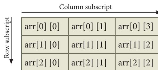
The array arr can be conceptually viewed in matrix form with 3 rows and 3 columns. The point to be noted here is since the subscript starts with 0 arr [0][0] represents the first element.
