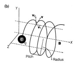
Component of velocity v parallel to magnetic field, will make the particle move along the field. Perpendicular component of velocity v, will cause the particle to move along a circular path in the plane perpendicular to the magnetic field. Hence, the particle will travel the helix path.
