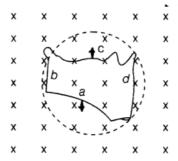
**Ans.** The wire is expanding to from a circle, which means that force is acting outwards on each part of the wire because of the magnetic field (acting in the downwards direction). The direction of the induced current should be such that it will produce magnetic field in upward direction (towards the reader). Hence, the force on the wire will be towards inward direction, i.e. induced current is flowing in anti-clockwise direction in the loop from cbadc.
