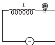
5. (a): In an A.C. circuit with inductance coil, the voltage  $V$  leads the current  $I$  by a phase difference of  $90^\circ$  or the current  $I$  lags behind the voltage  $V$  by a phase difference of  $90^\circ$ . Thus the voltage goes on decreasing with the increase in time as shown in the graph (a).
