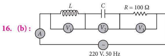
As  $V_L = V_C = 300 \text{ V}$ , therefore the given series LCR circuit is in resonance.
