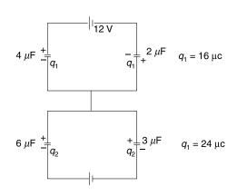
**19.** Capacitance between A and B is
