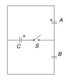
**Q. 36:** In the circuit shown in the Figure, find the ratio of potential difference across capacitor 1 and 2. The capacitance values are as indicated in the Figure.
