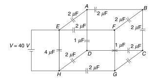
Points A and F can be joined together and points D and G can be put together. We can redraw the circuit as shown below.
