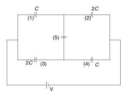
**Q. 37:** In the circuit shown in the figure, find charge on each capacitor.
