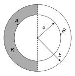
**Q. 32:** Two concentric spherical shells have radii a and b (>a). Write the capacitance of the system in following cases.
