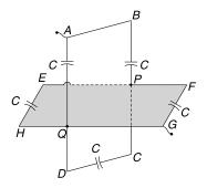
**Q. 17:** In the circuit shown in the Figure find the ratio of equivalent capacitance between A and B to that between A and C.
