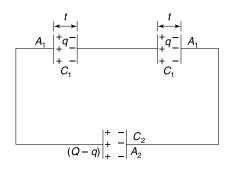
Let charge on capacitors having capacitance  $C_1$  be q and that on capacitor of capacitance  $C_2$  be Q-q.
