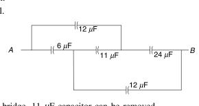
This is a balanced whetstone bridge. 11  $\mu$ F capacitor can be removed.
