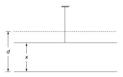
**Q. 49:** Two identical metal plates with area A and mass m are kept separated by help of three insulating springs as shown in the Figure. The equilibrium separation between the plates is  $d_0 (<< \sqrt{A})$  and force constant of each spring is K. When a constant voltage source having emf V is connected to the plates, the equilibrium separation changes to d. Assume that the lower plate is fixed and the upper plate is free to move.
