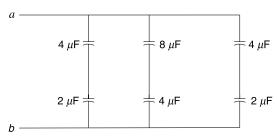
(b) With switch closed the circuit is as shown below.
