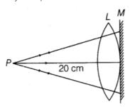
Since, the image is coinciding with the object itself, the rays from the object after refraction from the lens fall normally on the mirror M and form an image coinciding with the object itself. So, the image is formed at the focus of the lens. So, focal length of the lens is 20 cm.
