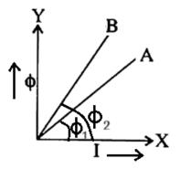
For two coils A and B, the diagram between magnetic flux and electric current is shown. Self-inductance of the coil will be more. Answer with proper reason.
