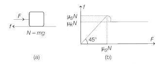
In Fig. (a), a force F is applied on a block of mass m. Force of friction f starts acting on the block in opposite direction to stop its relative motion with ground. Following cases may arise depending on the value of F.
