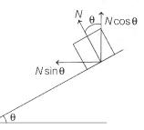
• Net contact force (F) can have two components, **friction** (f) which is tangential and **normal reaction** (N). Thus, N acts towards the body. Further N and f are in mutually perpendicular directions, hence
