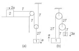
In Fig. (a), tension force on block-1 is double (=2T) the tension force on block-2 (=T). Therefore, acceleration of block-1 will be half.
