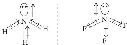
Resultant dipole moment in  $\text{NH}_3 = 4.90 \times 10^{-30}$  cm      Resultant dipole moment in  $\text{NF}_3 = 0.80 \times 10^{-30}$  cm
