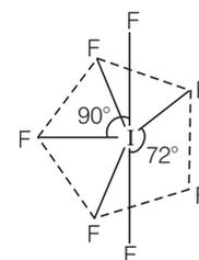
The structure of  $\text{IF}_7$  is pentagonal-bipyramidal.
