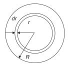
Considering an elemental ring of thickness 'dr' shearing resistance of the ring =  $q2 \pi r dr$ .
