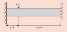
The maximum shear stress in the shaft is [GATE, 2009]
