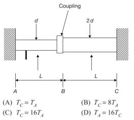
**3.** A shaft is subjected to torsion as shown in the following figure:
