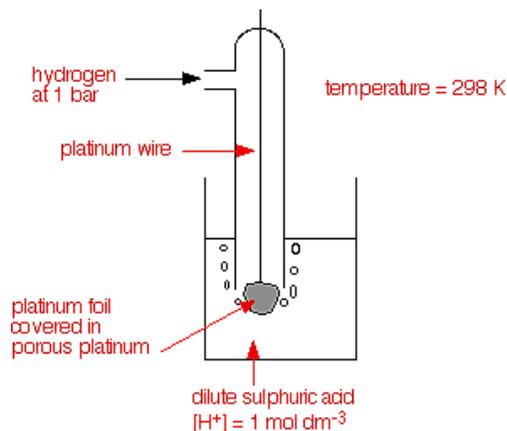
The electrode is immersed in an acidic solution and the pure hydrogen gas is bubbled through it.
