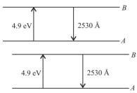
First they were excited to level  $\emph{B}$  and then thec atoms emitted spectral lines of 2530 Å i.e. 4.9 eV, Bohr's concepts were verified.
