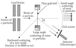
Schematic arrangement of the Geiger-Marsden experiment
