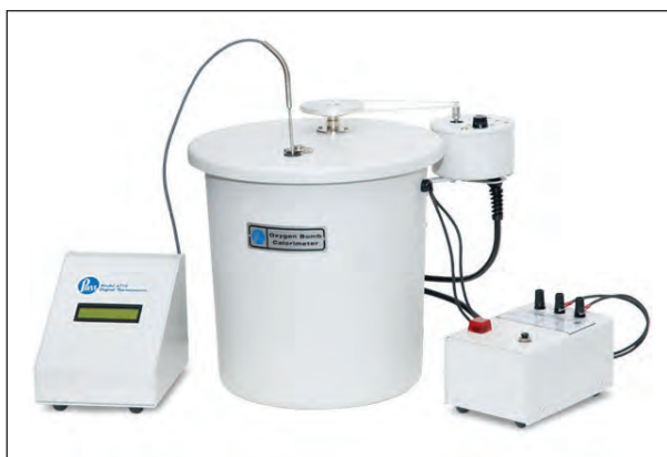
Figure 5.1 : Diagram of bomb calorimeter
