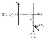
$$y = \frac{1}{2} \left( \frac{qE}{m} \right) \left( \frac{d}{V_0} \right)^2$$
