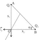
Net field along AB at O must be zero  $E_{\alpha}\cos\alpha = E_{\alpha}\sin\alpha$
