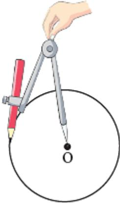
**Step 3:** Place the steel end of the compasses on the dot marked O. Hold the head of the instrument between the thumb and the forefinger such that the pencil end of the compasses may touch the paper. Now, turn it completely round so that the pencil end traces a circle. You will get a circle of radius 3 cm, with centre O.
