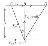
The component of velocity of boat parallel to the flow of water is  $V_{BR} \sin \theta$
