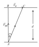
If  $\overline{V}_{BR}$ ,  $\overline{V}_{R}$  are the velocities of a boat and river flow respectively then to cross the river in shortest time, the boat is to be rowed across the river i.e., along normal to the banks of the river.
