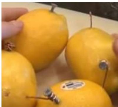
Step 4: Now connect an LED bulb to one end of copper wire and another end of zinc nail.
