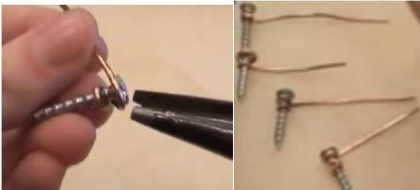
Step 2: Once all the nails are connected to the copper wire, we will connect each lemon to each other by screwing the nails.
