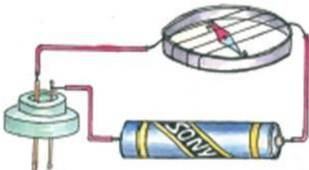
**Answer :** Yes we can avoid LED and use something else as a tester. Magnetic compass needle can be used as an alternative tester.
