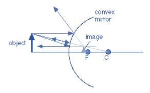
It is a spherical mirror which when looked from the reflecting side bulges at the center and is depressed at the edges.
