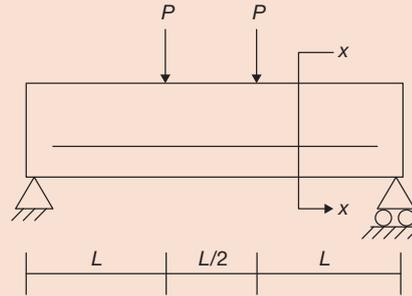
At cross-section x-x which of the following statements is TRUE at the limit state? [GATE, 2015]
