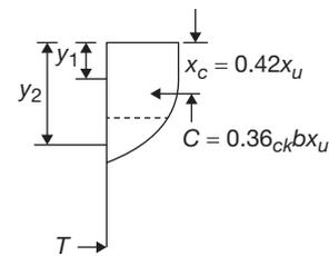
$y_1$ : Centroidal distance of rectangular portion from top compressed fiber
