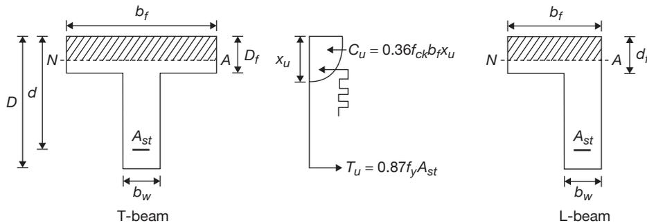
When neutral axis is within flange, the flanged beam can be treated like a rectangular beam of width  $b = b_f$ .
