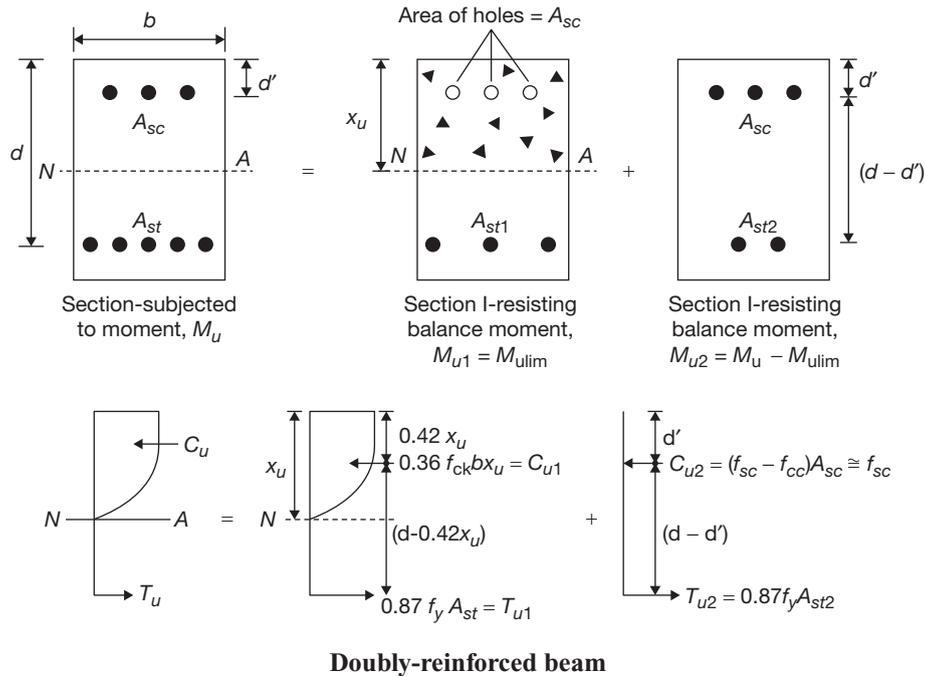
Moment of resistance of doubly-reinforced beam ( $M_u$ ) = (A singly-reinforced section with  $M_{ulim}$ ) + (A section with compression steel and additional tension steel to resist additional moment  $M_{u2}$ )
