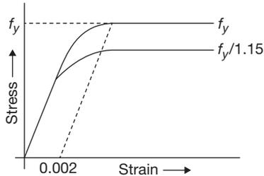
(a) Cold worked deformed bar
