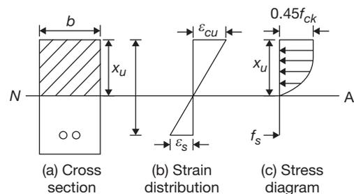
2. At limiting state, the maximum strain in concrete, which occurs at outermost compression fiber is 0.0035.
