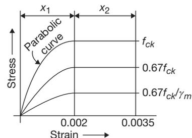
Idealised stress strain curve for concrete
