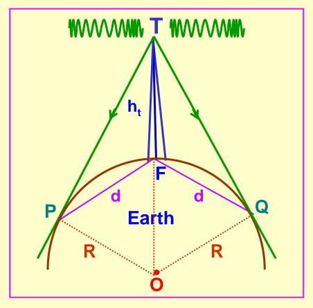
Let h be the height of the transmitting antenna, d be the distance (radius) of coverage from the foot of the tower and R be the radius of the earth.
