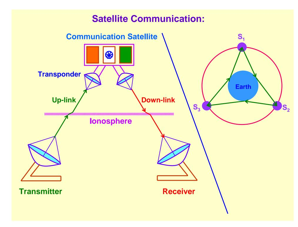
Satellite communication uses UHF / Microwave regions. Microwaves carrying audio, video, telephone, telex, FAX signals, etc. are transmitted from the earth to the satellites orbiting in the space and retransmitted from the satellites to different parts of the earth (world).
